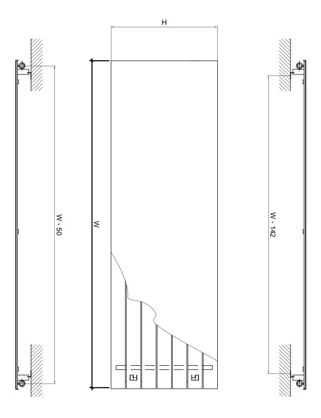
All dimensions in mm (W = width, H = height, NA = axial dimension between thread) Caution: maximum operating pressure 4 bar
