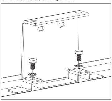
Place roof bars onto the roof brackets with the t-slot facing upwards, secure using top hat brackets, M6x16 coach bolts & M6 serrated nuts.
