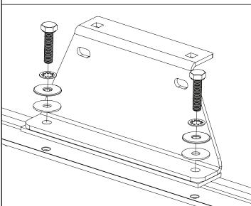
Place roof bars onto the roof brackets with the t-slot facing upwards, secure using top hat brackets, M6x16 coach bolts & M6 serrated nuts.
