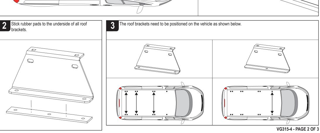
Secure roof brackets to the vehicles fixing points using M6x25 hex bolts, M6 shakeproofs, M6x20 washers & rubber washers. Ensure that the top hat flange is facing inwards.
