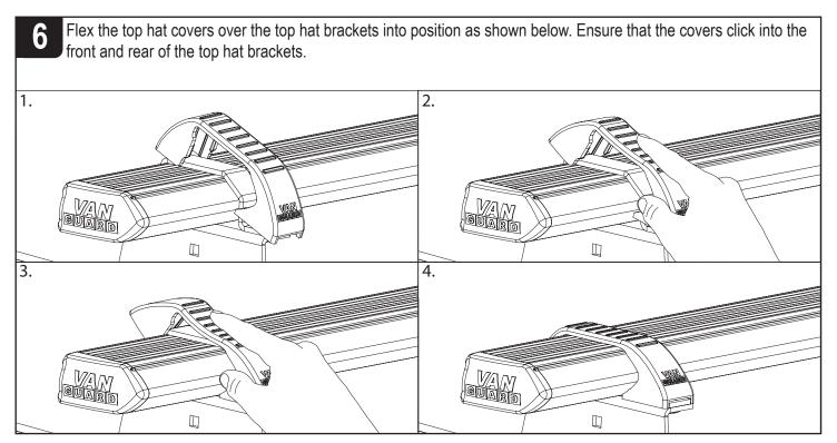
Once in position tighten all M6 fixings to 8Nm and all M8 fixings to 12Nm. Periodically check all fixings.
