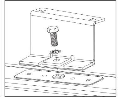
Place roof bars onto the roof brackets with the t-slot facing upwards, secure using top hat brackets, M6x16 coach bolts & M6 serrated nuts.
