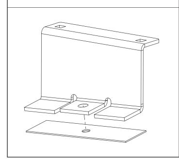
Secure roof brackets to the vehicles fixing points using M8x20 hex bolts & M8 shakeproofs. Ensure that the top hat flange is facing inwards.
