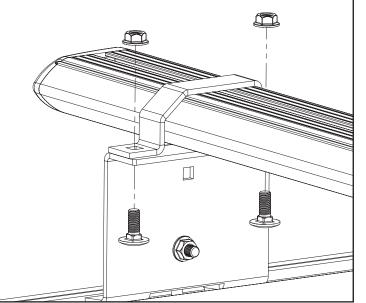
Flex the top hat covers over the top hat brackets into position as shown below. Ensure that the covers click into the front and rear of the top hat brackets.
