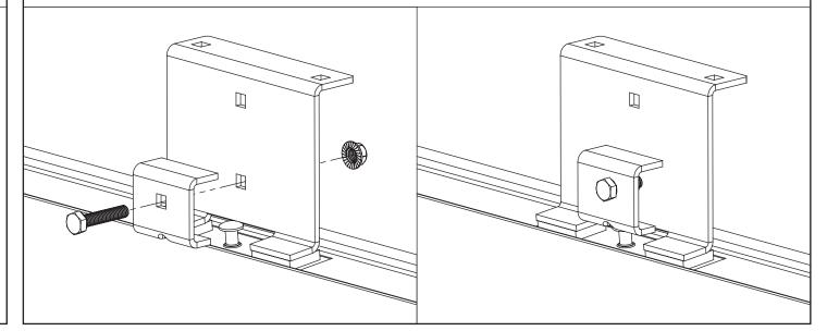
Place roof bars onto the roof brackets with the t-slot facing upwards, secure using top hat brackets, M6x16 coach bolts & M6 serrated nuts.
