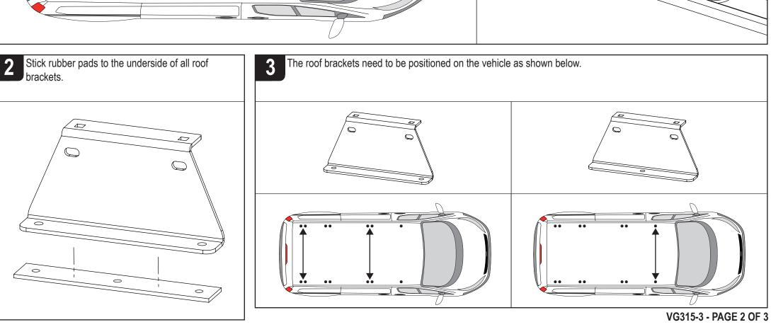
Secure roof brackets to the vehicles fixing points using M6x25 hex bolts, M6 shakeproofs, M6x20 washers & rubber washers. Ensure that the top hat flange is facing inwards.
