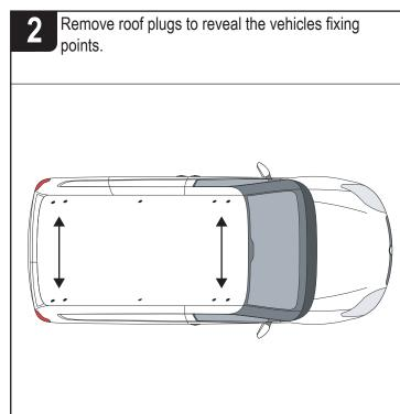
Secure roof brackets to the vehicles fixing points using M6x16 hex bolts, M6 shakeproofs & rubber washers. Ensure that the top hat flange is facing inwards.
