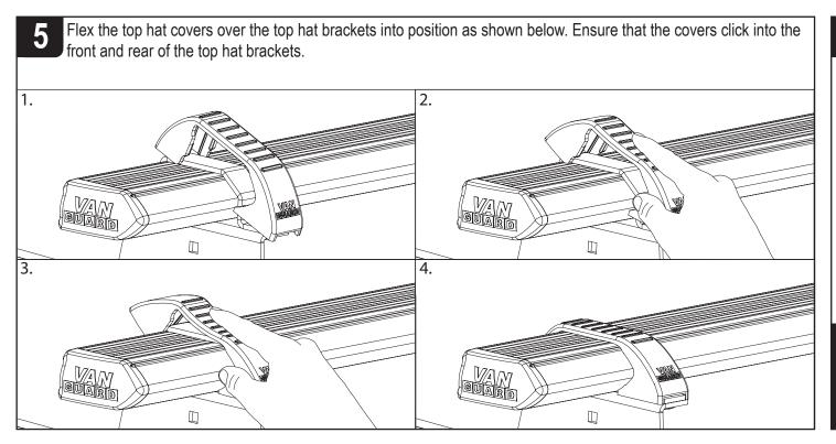
Once in position tighten all fixings to 8Nm. Periodically check all fixings.
