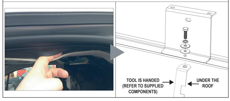
Place roof bars onto the roof brackets with the t-slot facing upwards, secure using top hat brackets,
