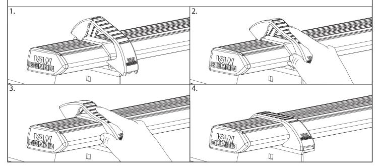
Once in postion tighten all fixings to 8Nm. Periodically check all fixings.
