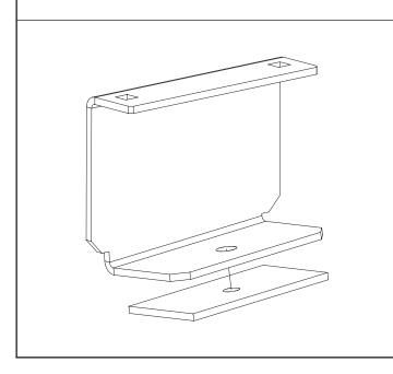
Secure roof brackets to the vehicles fixing points using M8x20 hex bolts, M8 shakeproofs & rubber washers. Ensure that the top hat flange is facing inwards.
