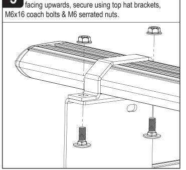
Place roof bars onto the roof brackets with the t-slot
