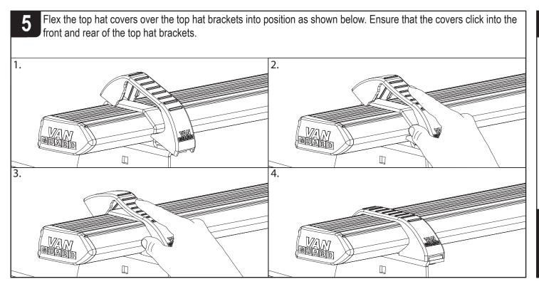
Once in position tighten all fixings to 8Nm. Periodically check all fixings.
