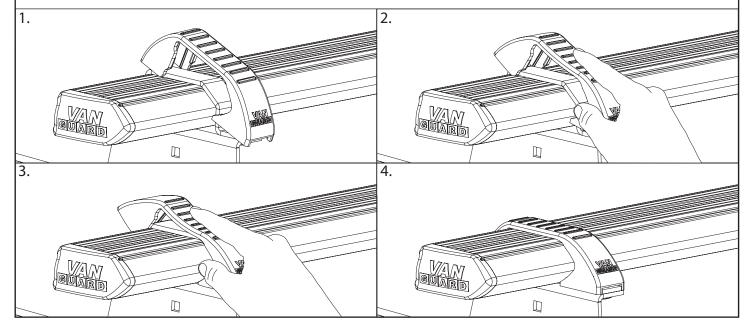
Once in postion tighten all fixings to 8Nm. Periodically check all fixings.
