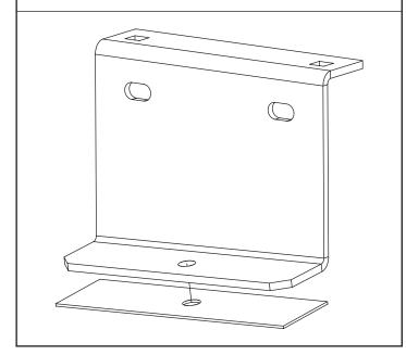
Secure the rear roof brackets by bolting through the vehicles fixing points using M6x30 hex bolts, M6x20 washers & rubber washers. Secure under the roof using M6x25 washers & M6 serrated nuts. Ensure that the top hat flange is facing inwards.
