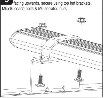
Place roof bars onto the roof brackets with the t-slot
