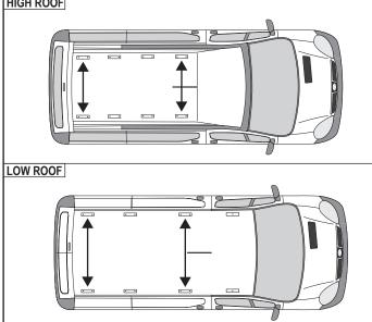
Secure roof brackets to the vehicles fixing points using M6x10 hex bolts & M6 shakeproofs. Ensure that the top hat flange is facing inwards.
