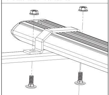
Flex the top hat covers over the top hat brackets into position as shown below. Ensure that the covers click into the front and rear of the top hat brackets.
