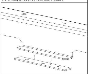
Remove roof plugs to reveal the vehicles fixing points. **Do not remove the front most roof plug as this is not required.**
