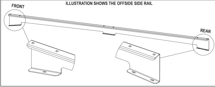
Stick rubber pads to the underside of the side rail feet. Please note, the middle foot of the side rail is for support only and is not secured to the vehicle. No drilling is required to fit this product.
