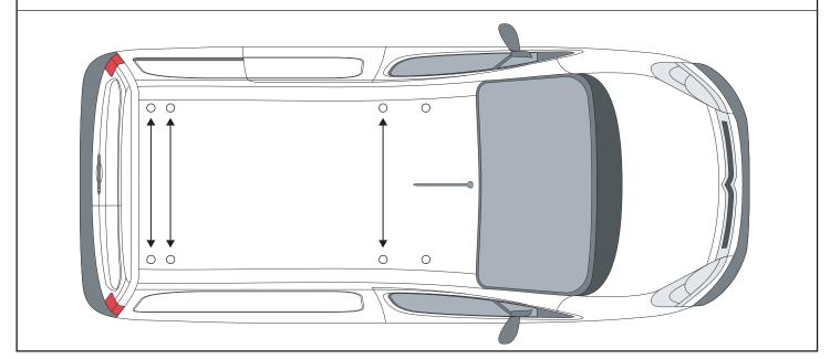
Secure side rails to the vehicles fixing points using M6x25 hex bolts, M6 shakeproofs, M6x20 washers & rubber washers. Ensure that the top hat flange is facing inwards.
