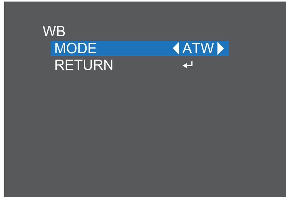
**ATW (Automatic White Balance):** The camera sets the White Balance according to the light it receives. We recommend you use this setting in most circumstances.
