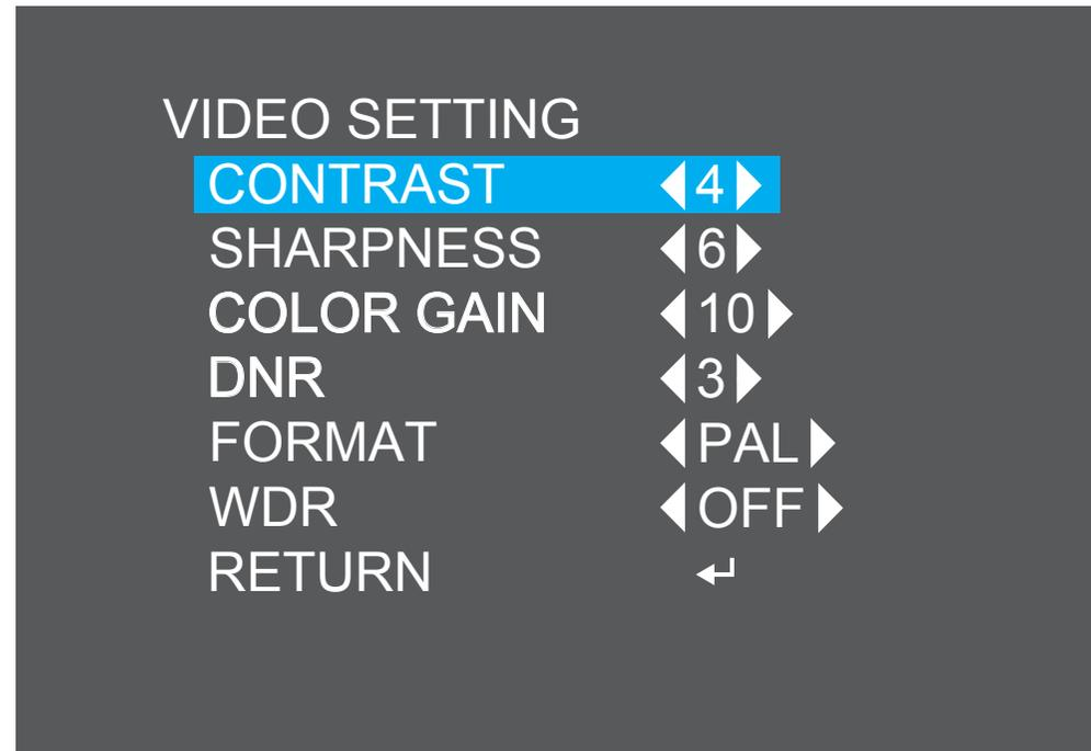
**Format (PAL-NTSC):** The reason for this option is mainly for indoor mounted cameras. Artificial lighting flickers slightly at the frequency of mains power which the cameras are able to see and shows on your screen as a flickering image. The correct setting here will eliminate any flicker produced by artificial lighting. For USA and Canada select NTSC, for AU, UK and most of Europe select PAL.
