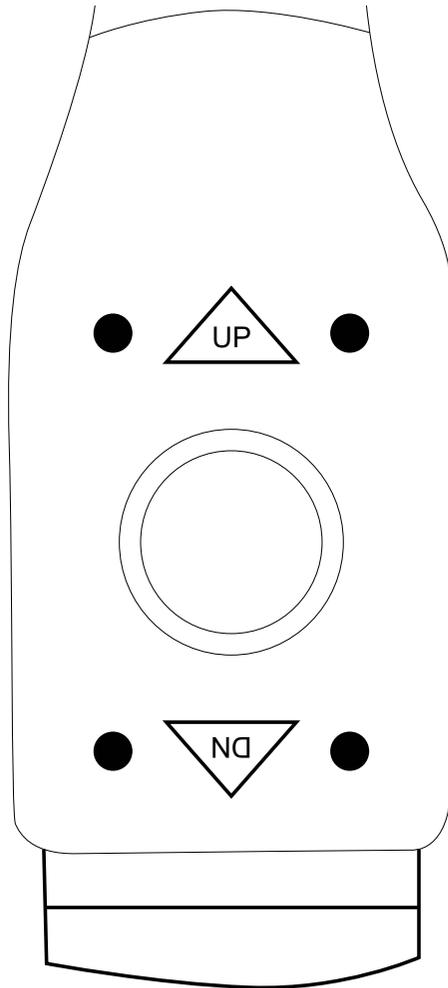
This camera has a joystick control on the cable connection to allow you to configure the camera settings to suit your DVR signal. The joystick is a simple 4 way stick configuration (up and down are noted on the fascia) and pressing in on the top of the stick is used to open the on-screen menu and as the 'Enter' key while in the OSD menu.
