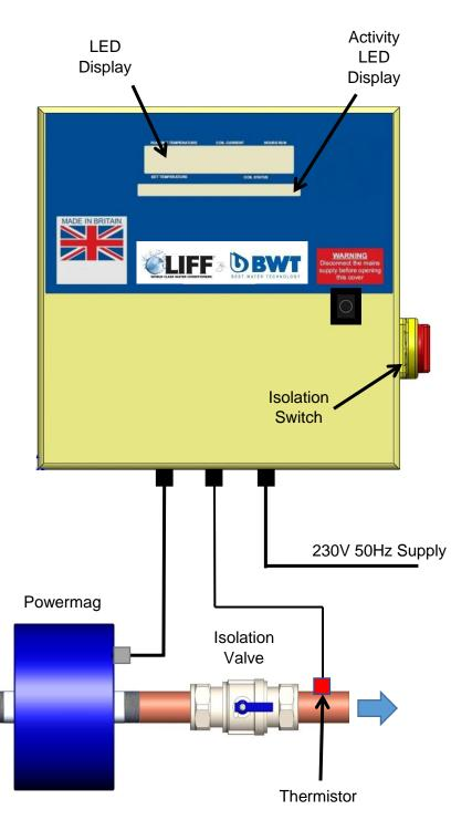
Powermag coil flying lead length supplied: 4.5m (approx.)
