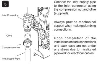
Always provide mechanical support when making plumbing connections.
