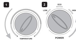
Turn temperature control to the Turn power control to low cold position.
