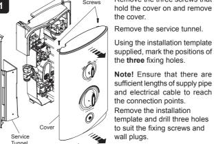
Caution! Do not drill into cables or pipes in the wall.
