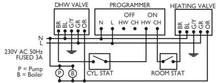
Typical circuit showing two 22mm two-port valves in fully-pumped systems
