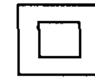
Your DeWALT tool is double insulated in accordance with EN 50144; therefore no earth wire is required.
