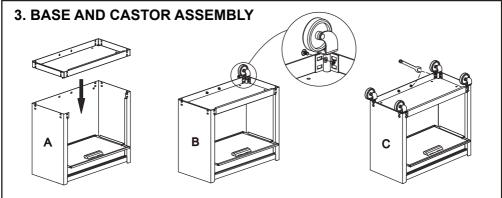
The bolts, nuts and washers need to be fixed by wrench, wrench not included.
