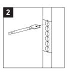
**2.** Between the lines for top and bottom of lock, mark a vertical guideline central to the door edge, to use as a guide for a series of holes to be drilled to the required depth.
