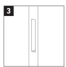
**3.** Chisel out the remaining wood to provide satisfactory clearance for the lock body (and intumescent material if fitting to a fire door). The mortice should be smooth and any shavings or swarf must be removed.
