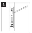
**4.** Insert the lock body into the morticed hole. Place the loose faceplate over the fixed forend, temporarily screw the faceplate on and mark around the faceplate. Remove lock from door and chisel out a recess to accept the complete depth of forend and faceplate (plus intumescent material if fitting on a fire door). Ensure any swarf is removed from mortice.
