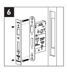
6. Ensure the mortice is free of any swarf and insert the lock into the mortice. Pre drill the forend fixing holes for screws and secure the lock in place. Fit the loose faceplate. Check that the Key/Cylinder and Spindle fit within prepared holes and that they operate the lock correctly. Additional levers and escutcheons can be fitted at this time. Test the final fitting to ensure the latch and/or deadbolt operate correctly.
