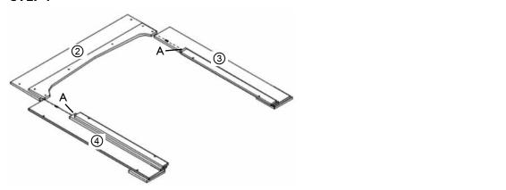
Lay the left leg(3) and the right leg(4) along with the front panel (2) on a soft floor. Next insert a 20mm dowel joint (A) into the top of each leg with a small amount of glue (J).
