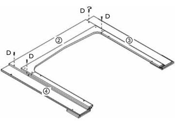
hand legs using the 4x25mm screws (D).
