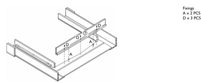
Install top inside panel (7) by attaching 2x dowels (A) to the front panel with the use of glue. Next screw 3x 25mm screws securing the top inside panel to the front panel.
