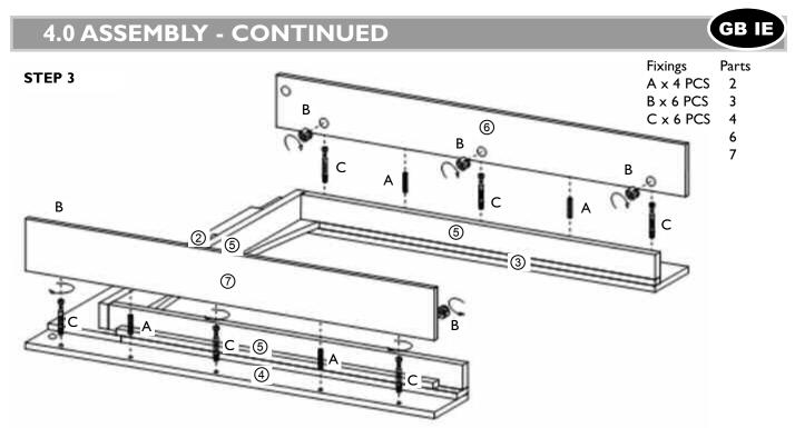
Use the Glue (I) in the dowel holes before inserting 2x dowels (A) into the left and right hand legs (3 and 4). Position the cam bolts (B) in to left and right side panels (3 and 4).
