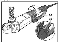
The main handle **34** can be rotated with respect to the machine housing toward the left or right in steps of 90°. In this manner, the On/Off switch can be brought into a more convenient position for special working situations, e.g., for cutting operations using the cutting guide with dust extraction protection guard **18** or for left-handed persons.
