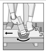
The machine must always work in an upgrinding motion. Otherwise, the danger exists of it being pushed uncontrolled out of the
