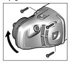
The machine head can be rotated with respect to the machine housing in 90° steps. In this manner, the On/Off switch can be brought into a more convenient position for special working situations, e. g., for cutting operations using the cutting guide with dust extrac-
