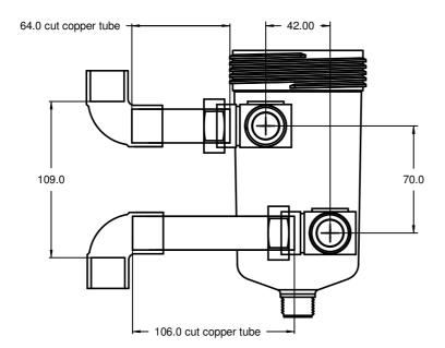
The inlet and outlet isolation valves should face the wall for a compact installation. The diagram shows how to mount the filter on the left of the pipe-run (looking from the wall). To mount the filter on the right of a pipe run simply swivel the isolation valves through 180° and swap the 106mm length to the upper position and the 64mm length to the lower position.
