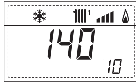
11. Display of number of times the burner has ignited x 1000 (eg 97000 and 500)
