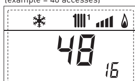
16. OEM access counter (example = 48 accesses)
