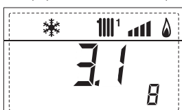
8. Display of ionisation current in \mu\text{A}
