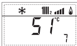
8. Display of ionisation current in \mu\text{A}
