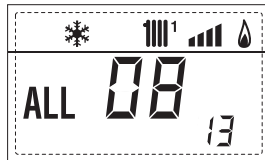
14. Display of total number of errors
