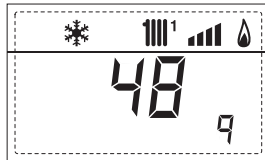
10. Display of the number of hours x100 the burner has been alight (eg 14000 and 10)
