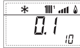
11. Display of number of times the burner has ignited x 1000 (eg 97000 and 500)
