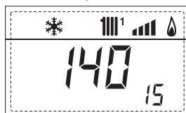
16. OEM access counter (example = 48 accesses)
