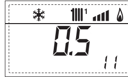
11. Display of number of times the burner has ignited x 1000 (eg 97000 and 500)
