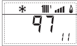
12. Display of code of last error
