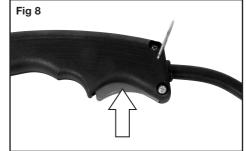
Do not point the end of the torch at any part of your body or face, the welding wire is very sharp and can cause an injury. When the wire has emerged from the end of the torch release the pressure on the trigger, turn the On/Off switch to the Off position then refit the contact tip and shroud. Finally trim off any excess wire to 3mm from the end of the contact tip.
