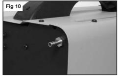
**Note:** shielding gas is not required when using flux cored welding wire.
