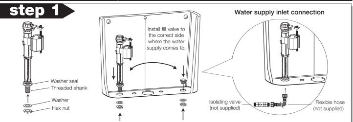
Ensure cistern is clean and dust free before installation. Unscrew the hexagon nut and washer from the threaded shank. Ensure the washer seal is attached to the threaded shank. Insert the fill valve into the cistern inlet hole vertically. Connect the washer and nut to the fill valve. Do not over-tighten but ensure fill valve is securely fixed, vertically positioned and will not interfere with the other mechanisms. Do not connect flexible hose or water supply until in its final position.
