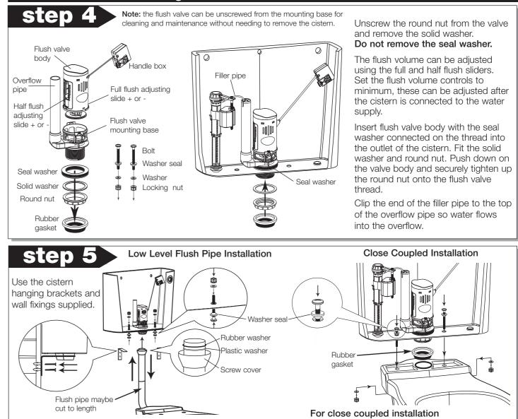
For low level installation. Connect the flush pipe together ensuring washer seals are tight. Connect the screw cover onto the flush valve thread on the outlet part of the cistern. Use the connecting bolts and washers to seal the bottom of the cistern. Note: the nuts and washers are on the inside of cistern. Ensure the washer seal is fitted correctly.
