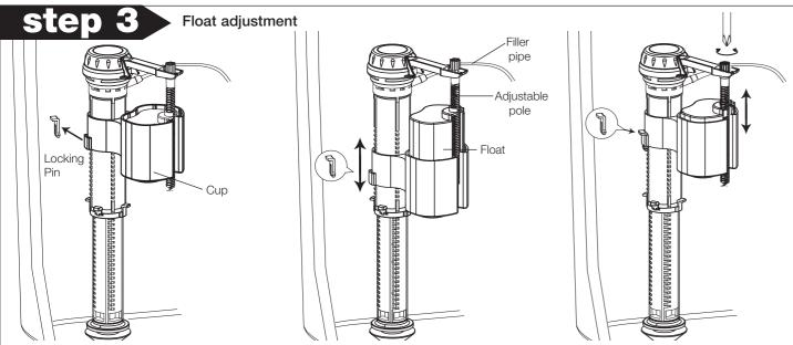
Take out the locking pin, adjust the height of the cup up or down depending on the water level required in the tank then re-insert the pin to lock in place. Note: the working water level is determined by the height of the top of the cup. Screw the adjustable pole to move the float up or down to the correct position so that the valve closes when the water is level with the top of the cup. Note that the non thread side of the adjustable pole should be facing outwards.
