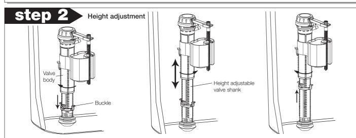
Unclip and push down the buckle. Lightly unscrew the adjustable body 1/4 turn anti-clockwise by hand and lift it up or down to an appropriate height between 20mm (8") and 300mm (12"). Turn the body clockwise until it clicks back into position and then lock the buckle back into its position to secure the valve body.
