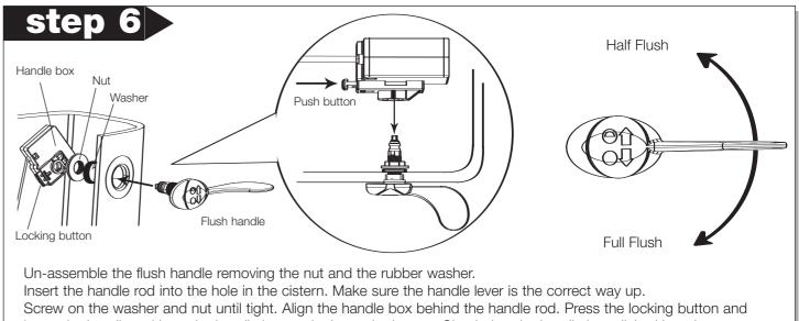
insert the handle rod in to the handle box and release the button. Check that the handle has clicked into the correct position and it has locked into place. Note: The handle can be installed on either side of the tank.
