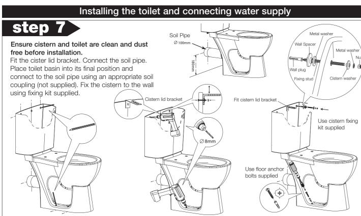
Fix the toilet to the floor. Use a plastic drill guide to protect the ceramic. For concrete floor installation use a suitable 8mm drill bit for drilling into the floor. Use 4mm to 4.5mm drill for wood floor installation. Install floor 10mm anchor bolts and cover caps. Do not over tighten the fixings as this can damage or break the ceramic.
