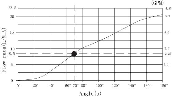
Flow diagram measurement tested at 3 bar.
