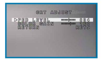
**PED LEVEL:** Altering the PED level will slightly alter the output voltage of the composite video out, altering the way that a CRT monitor will build images by combining the red, green and blue pixels on screen. Higher values will give brighter images, particularly in darker areas of greyscale. This is an expert feature – we'd recommend not touching it unless you know exactly what you're doing.
