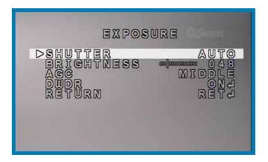
From the EXPOSURE menu, you can control how the camera reacts to lighting conditions.
