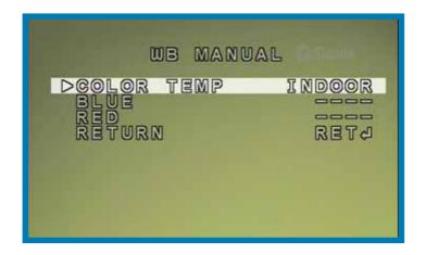
**COLOR TEMP:** Color temperature (technically measured in degrees kelvin) is a measurement of the average wavelength of light being photographed.
