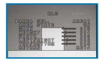
**AREA SELECT:** Choose which areas of the camera's view that you'd like to configure. You can have up to four areas defined and active simultaneously, which can overlap or be quite discrete.
