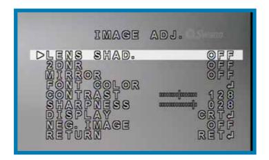
**IMAGE ADJ.:** The Image Adjustment menu allows you to control many aspects of the camera's pictures.
