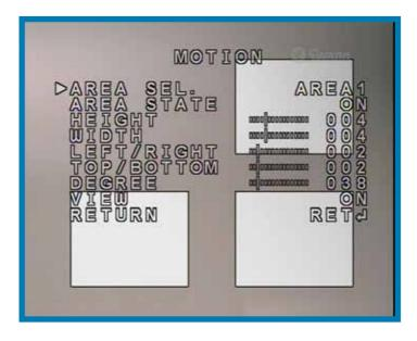
**AREA SELECT:** Choose which areas of the camera's view that you'd like to configure. You can have up to four areas defined and active simultaneously, which can overlap or be quite discrete.
