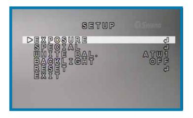
**Exposure:** Controls how sensitive the camera will be to light. Press SELECT to enter the Exposure sub-menu (page 9) to access the detailed exposure controls.
