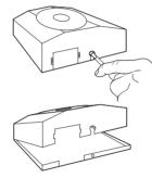
Standard cable entry is from the rear, but if surface wiring, from the top or bottom, is to be used, or extra space for cabling is required, use the optional Pattress box (sold separately).
