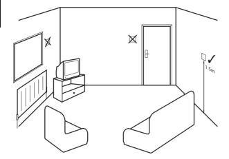
Care should be taken to mount the thermostat in a position which is not subject to direct sunlight or draughts. Preferably it should be mounted on an inside wall about 1.5m (5ft) above the floor in a position where it can respond to room temperature but away from the direct influence of radiators or other appliances giving off heat.
