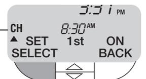
To change 1st ON time for CH press SELECT, time will flash, change times by using  $\triangle$   $\pm$   $\nabla$ , when desired time is in the display press ENTER display will show
