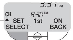
To change 1st ON time for CH press SELECT, time will flash, change times by using  $\triangle$  +/-  $\nabla$ , when desired time is in the display press ENTER display will show
