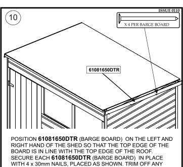
EXCESS FELT THAT IS SHOWING BELOW THE BOARDS.
