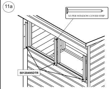
ATTACH EACH OF THE THREE **50120495DTR** (WINDOW COVER STRIPS) TO THE OUTSIDE OF THE SHED WITH 3 x 30mm NAILS. THE CENTRAL **50120495DTR** (COVER STRIP) SHOULD HAVE AN EQUAL OVER HANG ON BOTH THE LEFT AND RIGHT SIDE OF THE CENTRAL WINDOW BATTEN. THE OTHER TWO **50120495DTR** (COVER STRIPS) SHOULD BE PLACED FLUSH WIT THE OUTER EDGES OF THE CLADDING.
