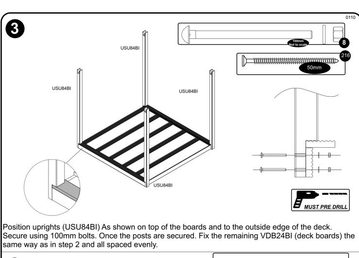
Secure using 100mm bolts. Once the posts are secured. Fix the remaining VDB24BI (deck boards) the same way as in step 2 and all spaced evenly. You may need to cut some components to the required length.
