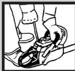
**2** Engage the chain brake by pushing the guard forward from the front handle.
