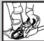
**7** When the engine fires cancel the choke by pressing the throttle lever and throttle interlock.
