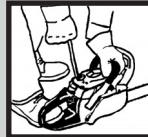
**9** Disengage the chain brake by pulling it back towards the handle.
