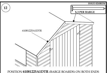
POSITION 61081225A1DTR (BARGE BOARDS) ON BOTH ENDS OF SHED SO THAT THE TOP EDGE IS IN LINE WITH THE TOP EDGE OF THE ROOF AND THE POINT OF THE 61081225A1DTR (BARGE BOARD) MEETS UP WITH THE HIGHEST POINT OF THE ROOF. SECURE EACH 61081225A1DTR (BARGE BOARD) IN PLACE WITH 3 x 30mm NAILS PLACED AS SHOWN ABOVE. TRIM OFF ANY EXCESS FELT THAT IS SHOWING BELOW THE 61081225A1DTR (BARGE BOARDS).
