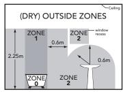
This product is specially designed for installation in a bathroom. It is IP65 rated and can be fitted in Zone 1, Zone 2 and Outside (dry) zones of a bathroom - see diagram left. The bezel on this product provides the IP65 protection. The electrical parts of this product must be installed in a fully enclosed ceiling void with the bezel fitted to maintain the IP65 rating.
