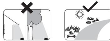
Avoid locations where light from other sources will fall on the panel at night (street lights etc) as this may prevent the light from turning on.
