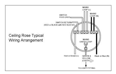
7. Connect the supply wires to the terminal block, opposite the corresponding wires from the fitting. See opposite. Ensure that connections are tight and no loose strands of wire are left out of the connector blocks. This product must be earthed – if no earth feed wire is available, consult an electrician.
