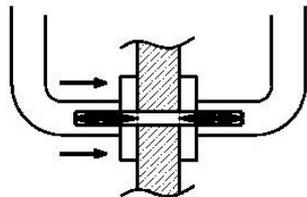
Insert spindle through lock/latch follower ensuring that lever is correct way up in respect of design and spring action, so that the inner rose is flat against the face of the door.
