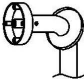
Remove outer rose and slide carefully off, ensuring not to damage the lever finish in the process to view fixing holes.
