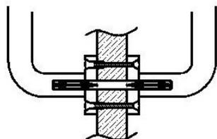
Insert male bolts through inner rose so they locate cleanly with female bolt from the other side. Tighten bolts ensuring threads do not cross. Replace the roses
