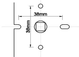
Handles can be bolted either vertically or horizontally with the fixings supplied. It is necessary to use locks and latches with a bolt through facility for horizontal fixings.
