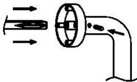
Locate spindle in one lever ensuring, if applicable that the spindle groove is aligned with the grub screw hole in the lever shank. Once lever is suitably aligned secure it in place with the grub screw provided, ensure there is sufficient spindle projection so it can be located in the other handle.
