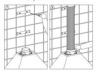
Mount upper and lower bracket (3, 4) on the wall. Secure with the remaining 4 sets of long screws (7) and wall plugs (8) (fig. ①).
