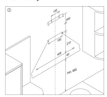
Using upper and lower bracket (3, 4) as a templates, mark and drill 4 holes in the wall (fig. ③). Screw and tighten the cooker hood onto the wall with 4 sets of long screws (7) and wall plugs (8).
