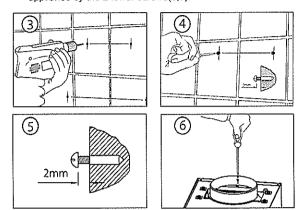
Attach the collar (4) to the cooker hood (1). Secure with 2 short screws (8) (fig. 6).
