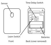
The Dusk to Dawn Sensor is designed to automatically turn on any LightwaveRF receiver, such as a bulb or dimmer, at dusk. The sensor will then automatically turn off devices again at dawn or after a specified delay period.
