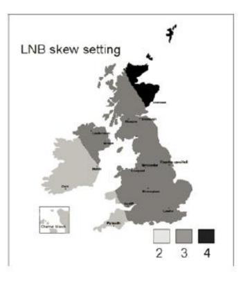
The three numbered zones on the map above indicate the required LNB skew setting for different areas of the UK and Ireland. These correspond to the numbers marked for the skew settings on the LNB. Note that only settings 2, 3 and 4 are relevant for this geographical area.
