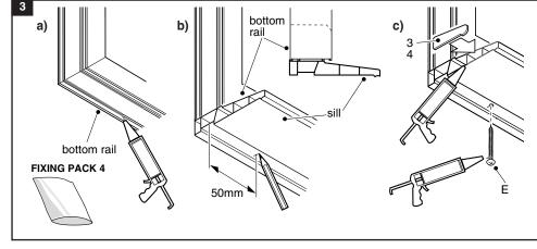
To ensure that the door operates smoothly it is vital that the frame is installed correctly. The frame MUST be fitted plumb and square. Check with a spirit level of adequate length, by measuring the frame corner to corner diagonally to achieve an equal measurement, or by using a square. It is also recommended that the door is checked for bowing by using a long straight edge.
