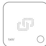
If pairing fails (E0), make sure the distance between the devices is approximately 3 meters. Pair again by pressing the button for 3 sec.
