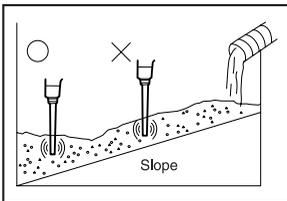
When concreting a slope site, always pour from the bottom at the beginning. This way the weight of the freshly poured concrete and vibration will lead to effective removal of air bubbles. Conversely, if the pouring is done first from above, the mortar will separate and eventually slide to the bottom.
