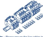
**Note:** - Please ensure the live cables to RCD1/RCD2 are fitted under the busbar in the main switch live terminal.
