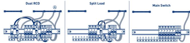
**Note:** - Terminal Bar 'A' is for optional high integrity, unprotected circuits.
