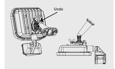
Fit floodlight to the wall using suitable fixings. Tilt and rotate floodlight to desired angle and securing fixing bolt. Ensure product is secure.
